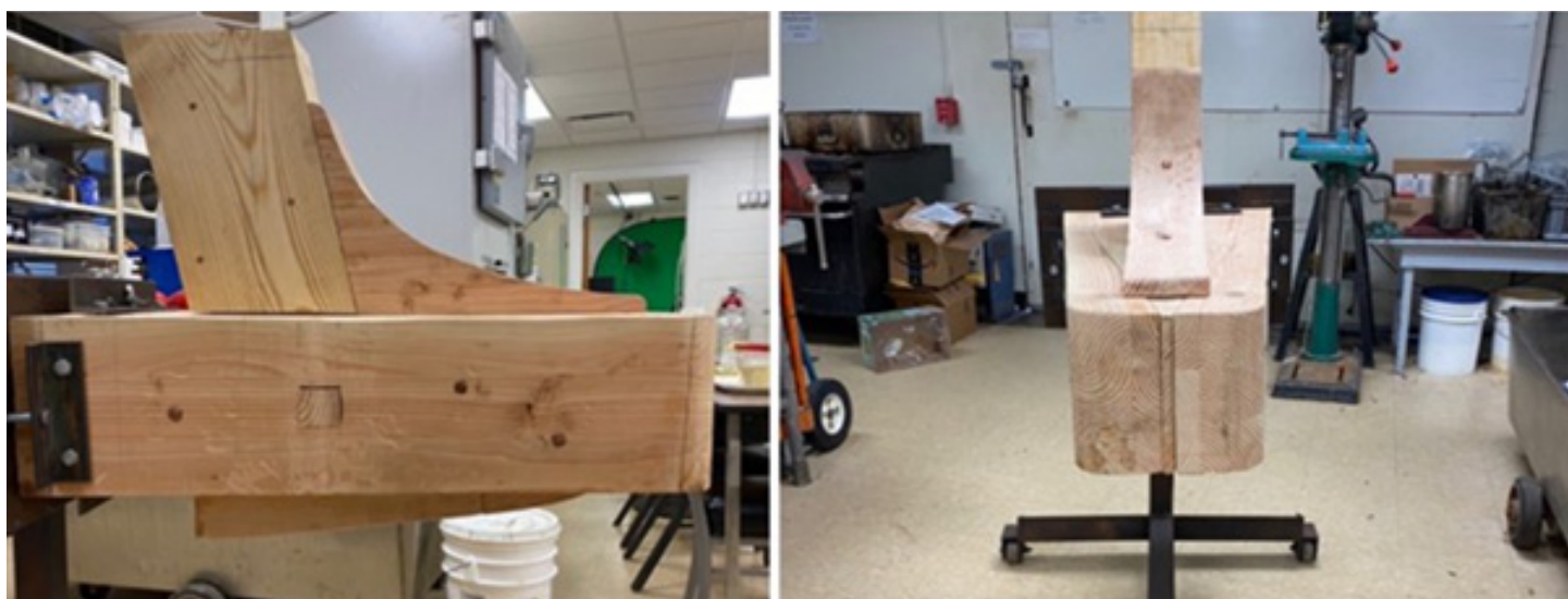
Figure 3: Fully constructed false trireme ramming bow. Photo by the author.
